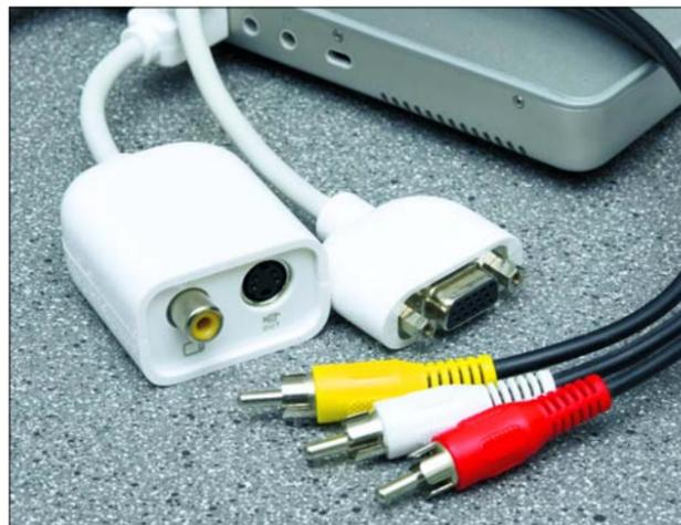
Laptops and desktops either come with connections for TV and projector use or an adapter will be supplied. This is an RCA adapter used with the tricolour RCA cables, though only one cable is necessary. The other is a VGA adapter for projector use.
