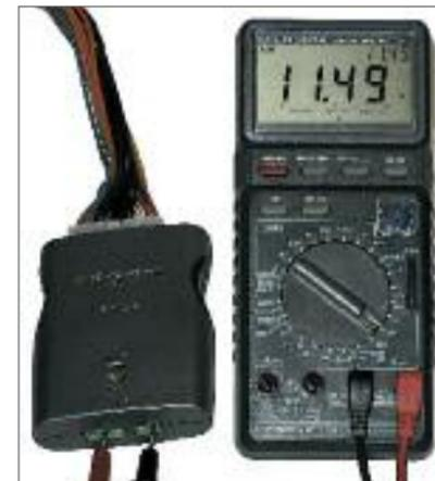
As a last resort, try using a relatively cheap and handy voltmeter. You can check to see if a particular wire is broken or has corrosion that reduces current flow.
