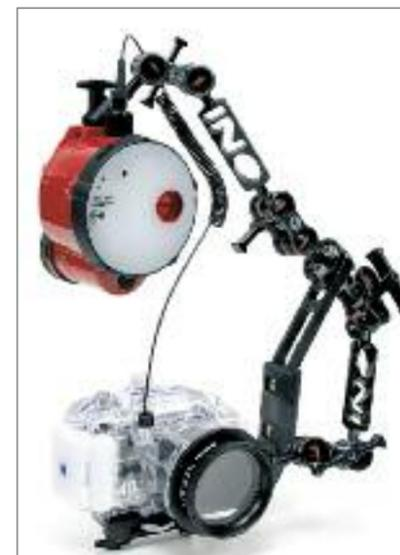
A typical housing/strobe setup. This one is particularly interesting because the connectors are optical and the sync cable is an optical fibre. The strobe reacts to a tiny light pulse fired by the camera via a small electrical component attached to the inside of the housing. Cleaning the optical contacts, cable tips and changing batteries is about all you can do here.
