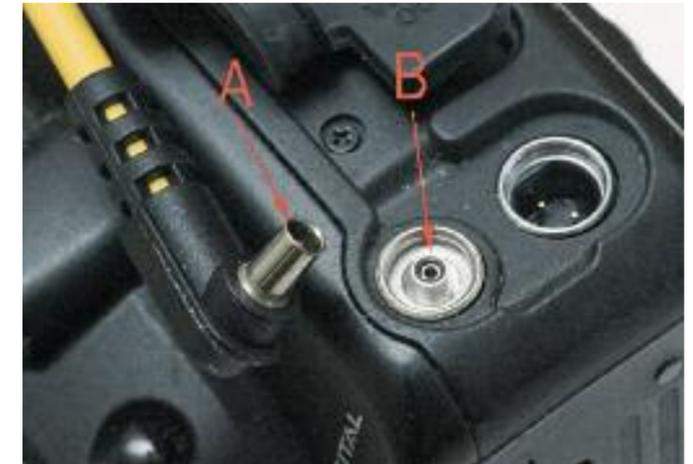
Hidden under a flap can be found my camera's sync socket (B) into which a right-angled sync nipple (A) can be inserted. The outer metal sleeve can be gently squeezed out of shape a tad to make a tighter fit, if that is a problem. If not, leave it alone. Inserting the nipple and twisting it around a few times is usually enough to make a secure electrical contact.
