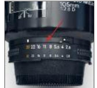
The standard f-stops are shown on this Nikon 100mm macro lens (A). f2.8, f4, f5.6, f8, f11, f16, f22 & f32. These are standard f-stops with the numbers representing apertures that let in half the light for each step as you go up the scale. Digital cameras will have either extra 1/2, or more often 1/3, stops as well.
