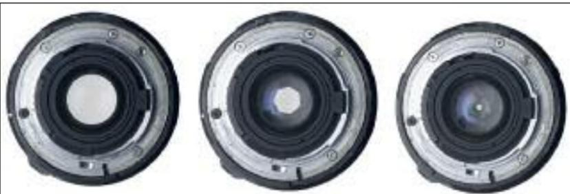
The aperture is a set of moveable metal sheets designed to produce a roughly circular 'hole' through which light has to pass to reach the sensor. This 60mm Nikon lens shows, from the rear element, an open aperture set at f2.8, a partly closed f8 and the minimum aperture of f32. The aperture is always set inside the lens body at a point where the light beams cross within the optical array of the lens. It is a more sophisticated version of dropping the visor in your car if the light is too bright.
