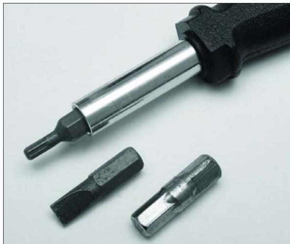
Lighten your baggage load by paring down on weighty objects. A multi-use handle can hold allen key, screw driver and phillips bits. Total weight is much less than all of the normal tools.
